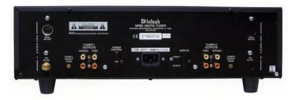
BACK PANEL: ANTENNA 1: external AM ANTENNA (RAA1) and 75  $\Omega$  FM ANTENNA coax input. TUNER 1 OUTPUT LEVEL control. Left & Right TUNER 1 VARIABLE and FIXED OUTPUTS. POWER CONTROL IN and OUT. Power cord receptacle. DATA IN jacks for TUNER 1 and 2. Left & Right TUNER 2 VARIABLE and FIXED OUTPUTS. TUNER 2 OUTPUT LEVEL control. Spaces reserved for optional TM 1 second tuner module: ANTENNA 2: external AM ANTENNA (RAA1) and 75  $\Omega$  FM ANTENNA coax input.
