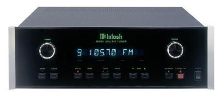
FRONT PANEL: Glass with illuminated teal/gold nomenclature. PRESET control. Digital readout: preset station tuned, frequency display, broadcast band and signal strength. FM stereo signal light. TUNING control. Push buttons: ENTER (with indicator), DISPLAY, SPATIAL (with indicator), MONO, TUNER 1 or 2, AM or FM, ▼ SEEK, SEEK A, AUTOMUTE (with indicator), STANDBY/ON (with indicator), POWER ON or OFF. Additional AM/FM TM 1 tuner is optional.
