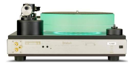
**BACK PANEL:** LEFT and RIGHT audio OUTputs. Ground connector. POWER CONTROL: REMOTE IN and REMOTE OUT. PLATTER LIGHT adjustment. SPEED CONTROL FINE ADJUSTMENT: 78RPM, 45RPM and 33-1/3RPM adjustments. DC IN 24 V connector.
